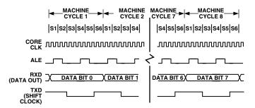
Figure 32. UART Serial Port Transmission, Mode 0
